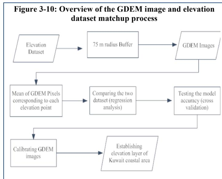
total of six GDEM images, each representing a 60 km by 60 km area of Kuwait, were downloaded and used in the process. GDEM elevations are expressed as the distance in meters above mean sea level.
